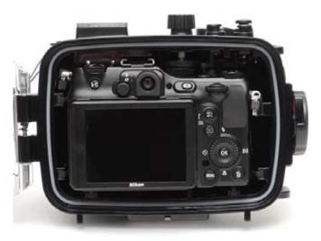
Loading the camera is a piece of doddle. Fantasea recommend removing the camera's strap lugs but in practice, if they are lifted up, they don't get in the way. Then all you have to do is lift the front mode dial and feed the camera into the front of the housing where it is held very precisely in 8 padded supports and four front posts. All but 3 of
